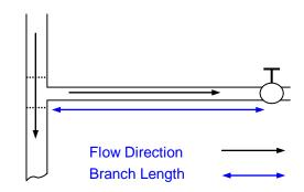
time the secondary barrier is the "Tee" itself. If water is flowing in the branch line and the valve is closed quickly, a shock wave will develop. Its inception follows the same sequence of events seen in our hypothetical example. One small difference is that some of the intensity of the waves will be lost in the "Tee" as it is open to the main pipe line on either side. Still, a significant portion will be reflected back towards the valve.
