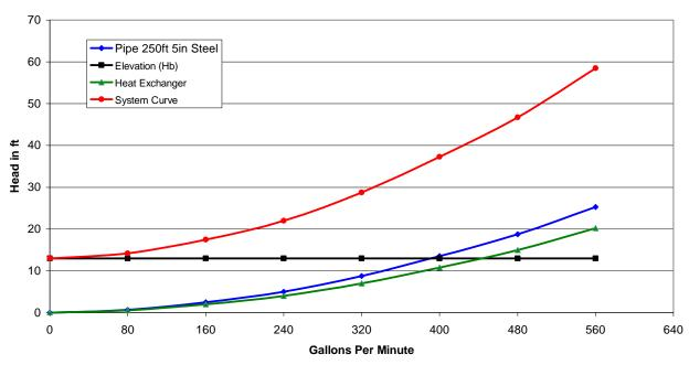
Open Loop Friction & Static Head
