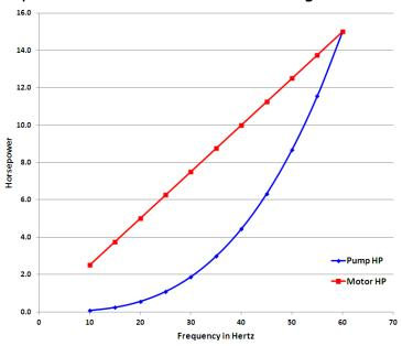
speed, power requirement of 15 HP. The ratio of available motor Hp to the required pump HP increases exponentially as speed is reduced. Figure 2 shows this relationship for the same pump and a 10 HP motor. In this example, available HP does not meet the required HP until speed drops below 50 Hz. If our reader's design point could have been met at 45 Hz, the 10 Hp motor would have been more than adequate.
