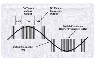
both the positive and negative portions of the AC cycle. The sum of the areas of the pulses equals the effective voltage of a true AC wave (we will discuss effective voltage in a few minutes). If you were to chop off the portions of the pulses above (or below) the true AC wave and use them to fill in the blank spaces under the curve, you would find that they match almost perfectly. It is in this manner that a VFD controls the voltage going to the motor.
