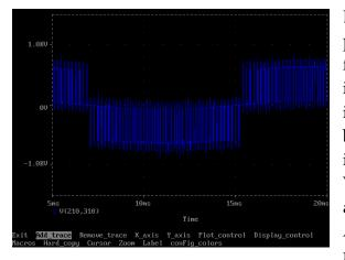
Eliminating the voltage spikes seen in the previous illustration can be as easy as following NEMA cable length guide lines or it could be more complex and require the installation of load reactors or dv/dt filters between the motor and the drive. The illustration to the left shows the same 460V VFD output after appropriate corrective action (cable length, filters etc) was taken. As you can see the 1500V spikes have been reduced to nearly that of the 650V pulses.
