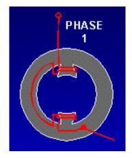
will cause the rotor of the two pole motor to complete a single rotation. If the AC frequency is 60 Hz the motor will rotate at 3600 RPM (60 rotations per second times 60 seconds). At 50 Hz the rotational speed will be 3000 RPM and at 30 Hz it will rotate at 1800 RPM.
