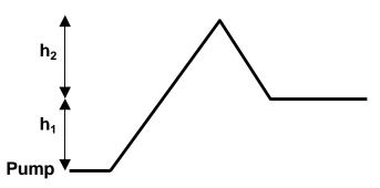
affect pump head is due to head recovery provided by the "siphon effect". Now, h2 must be accounted for when filling the line but, once it is flowing full the down leg will cancel its additional height and the elevation seen by the pump will be h1. If the down leg is not flowing full, the head required will be that of
