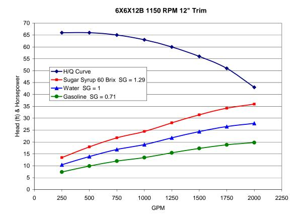
The downward sloping curve in the upper portion of the graph is the H/Q curve and the red, blue and green curves are the horsepower curves for three different liquids. The scale of the Y axis is both head and horsepower. The blue curve shows the HP required for water (SG=1). The red and green curves show the HP
