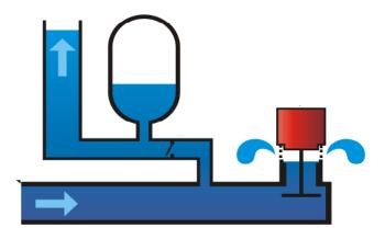
chamber. When the delivery check valve closes, the remaining water in the drive pipe recoils against it. This creates a low pressure area that allows the waste valve to reopen. And, as before, the cycle begins again.
