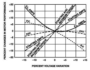
example, the graph shows that a 10% decrease in supply voltage will result in a 10% increase in current draw. As long as this increase does not exceed the nameplate current no damage will occur. In fact, on lightly loaded motors a small voltage drop can actually improve efficiency (the Nola effect). If, however, the motor is already loaded to its nameplate amperage, a 10% voltage drop will definitely have an adverse effect on motor life due to the additional heat that will be generated.
