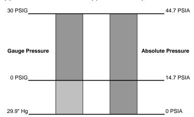
include atmospheric pressure and will read 14.7 PSI at sea level. Figure 1 compares these two pressure scales. On the absolute scale, 0 PSI equates to a perfect vacuum but on the gauge scale it equates to atmospheric pressure.
