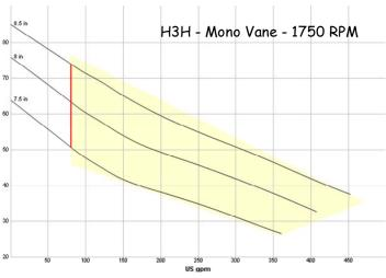
of heads and still pass a 3" spherical solid. This impeller design offers a viable alternative to off BEP operation of a two vane impeller.
