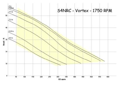
If you have lower flow applications that still require the passage of large solids, I encourage you to investigate these impeller alternatives. Lower flow, solids handling pumps are generally less efficient than higher flow models. Therefore reliability - not efficiency - should be your major concern.
