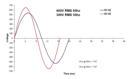
When frequency and the resulting motor speed is changed, the applied voltage is always changed in the same proportion. This allows magnetic flux and the torque it produces to remain constant regardless of speed. In the case of a 60hz motor running on 50hz power, voltage is reduced by 1/6. In the case of VFD control, that voltage is varied in proportion with every single change in frequency whether it be up or down.
