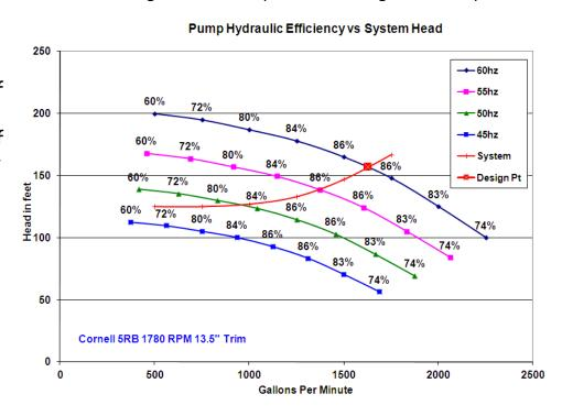
duty point head calculations as well as ageing of the system. It still performs at 85% from 1375 to 1875 GPM and will maintain 84% from 1250 to 1900 GPM.
