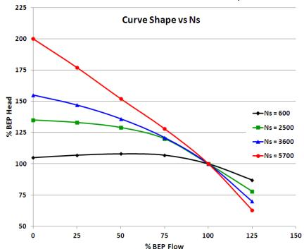
55% increase in head. The red curve (Ns=5700) is extremely steep and head increases by 100% from BEP to shut off. Steeper curves usually offer a greater range of control when operated under variable speed control against some fixed elevation or pressure head. Flatter curves work fine in across the line applications as long as the static or pressure
