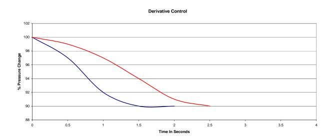
I said the feedback seen by the VFD is usually one dimensional but, that single source provides a continuous stream of information. Depending upon the processing power of the controller, it might be monitored anywhere from 5 to 10 times each second. Since the controller is continuously updated with new pressure information both the integral and derivative functions can drastically increase the accuracy of the proportional algorithm by providing it with real time guidance.
