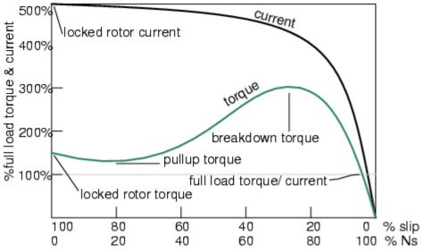
motor that speed is reduced to 1800 RPM. Slip or slip speed is the actual rotational speed of the rotor and it is typically 3 to 5% lower. The reason that an induction motor operates below synchronous speed is pretty simple. If the rotor were to move at the same speed as the rotating magnetic field in the stator there would be no relative motion between them. Therefore no flux lines would cut across the rotor bars and no magnetic field would be induced.
