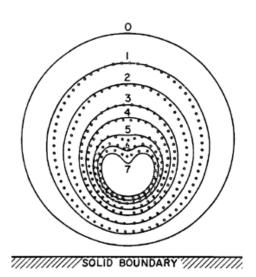
Upon implosion, the re-entrant micro jet would normally form at the bottom of the bubble and direct its energy towards the solid boundary.
