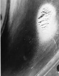
The two pictures on the left are of the same area of a centrifugal pump impeller. The one on the left shows a typical cavitation pattern during flow. Bubbles are forming to the left and imploding at the impeller's surface in the upper right. The picture on the right shows the actual damage caused by continuous implosion of bubbles in the same area.
