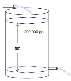
then the drain must have the same capacity if the level is to remain the same while both are operating. Since the flow rate is 2200 GPM it should take about 91 minutes to fully drain its 200,000 gallon capacity. No calculus needed here - - just basic arithmetic.
