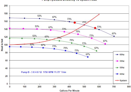
Pump Hydraulic Efficiency vs System Head
