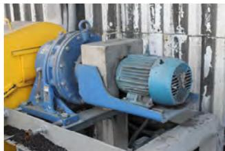
It would not be unexpected that many of the pumping applications in a pulp and paper mill could be difficult at best. Many of the pumps installed in sumps tend to clog frequently due to the content of the pumpage. Over the past three years, ten problematic systems have been replaced with Vaughan chopper pumps. These pumps can handle difficult applications without clogging.
