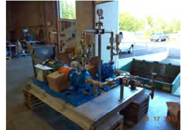
water treatment skids under construction for GE. These will be used in a water treatment facility that they are supplying for Panda Energy.
