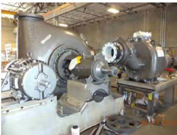
Goulds water pumps. The photos show several skids under construction plus some of the pumps, motors and base plates awaiting assembly. All of the base plates, coupling, and belt guards are 304 welded stainless steel.
