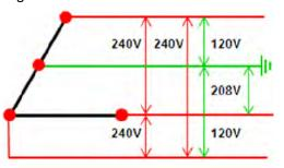
right. This design combines all of the weaknesses of the previous mutants. Not only is it subject to voltage unbalance due to the use of just two transformers, it also increases the probability of unbalance by providing two single phase connections on a single transformer. If this design powers a three phase motor and its single phase control circuit, it is always best to disconnect all other single phase loads.
