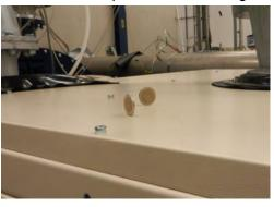
blowers installed and operating so they can begin saving energy as soon as possible. The various pictures show the HST's during testing. In the one above, two coins can be seen standing on edge. This illustrates that the HST's have virtually no vibration even when operating at 22,000 rpm!
