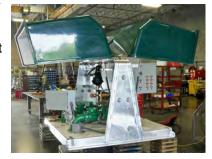
underground valve vault but it was decided that a Hydronix 430 series above ground combination valve and control vault would be a better fit for this particular application. A photo of the 430 during
