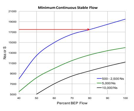
required to provide stable operation at or below 80% of BEP flow.
