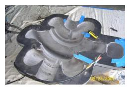
and those pits were filled prior to the coating process. Figure 4 shows the same pump after application of the metal filler and two coats ceramic filled, epoxy coating.
