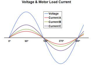
regardless of the motor load. It is often referred to as "reactive, imaginary or borrowed power" and it is not measured by a standard kWh meter because it is out of phase with voltage. Later we will see how the combination of varying load current and constant magnetizing current will cause power factor to vary from its nameplate value.
